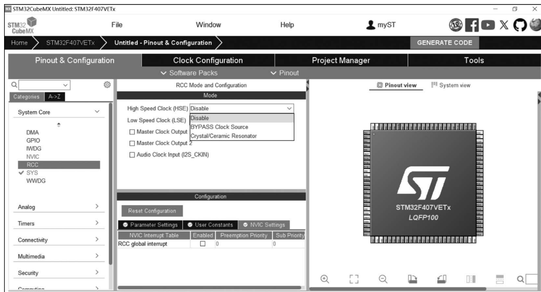
图 3-11 RCC Mode and Configuration
